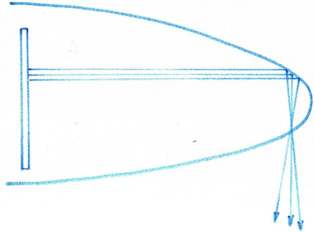
Fig. 5. Downward lobe from radome nose reflection
